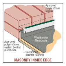
For masonry or brick veneer inside edges run the membrane up the required number of blocks to achieve the proper upstand. Make a saw cut into the mortar joint and insert a galvanized counter flashing. Both the membrane and flashing should be sealed in place with an approved polyurethane sealant. The flashing should extend down over the membrane a minimum of 50mm.
