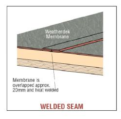
layers with a neoprene rubber roller. Weld approx 18" to 24" with this pass and then make a second pass over the weld to bevel the edge of the join.
