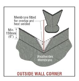
When gluing the membrane in place, adhere it tight to the deck surface and locate the point where the membrane will meet the corner of the wall. Make a 45° cut from this point back towards the wall and fit the membrane around the corner. Cut an over flashing made of Weatherdek membrane that will overlap the existing membrane by 1". Glue this piece in place and heat weld the overlaps.
