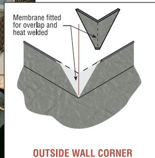
Laid out and fully adhered to most smooth substrates, Weatherdek membranes are heat welded at all joints creating a continuous layer of waterproofing protection.
